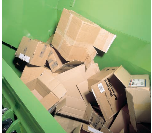
2. During the forward cycle the whole filling area remains available for continuous charging
