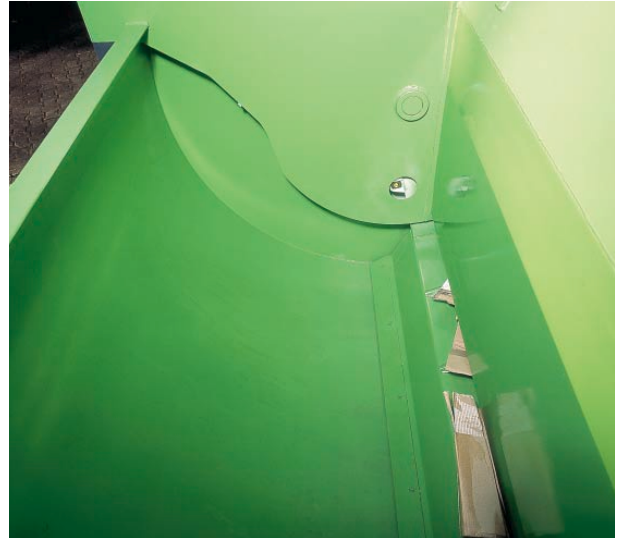
4. In the forward cycle the material is pressed under the breakwall into the box
