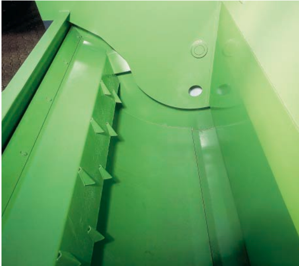
1. Illustration of the self-cleaning pendulum blade in the backward position
