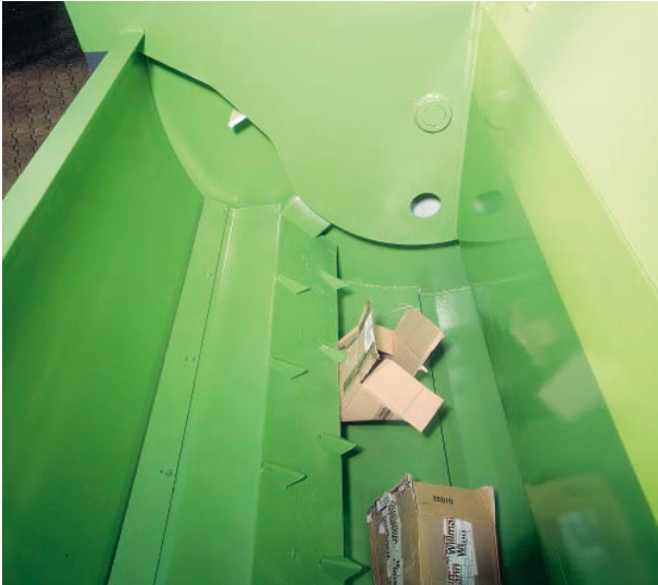
3. In the return cycle the pendulum blade passes under the material and pushes it in front of itself
