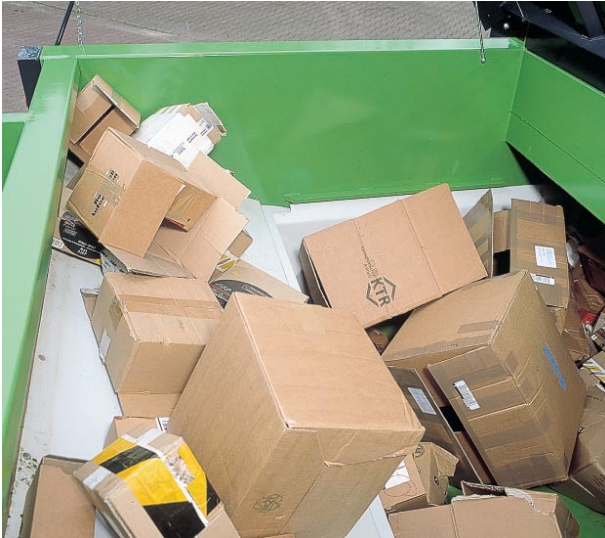
3. In the return cycle the throw-over blade passes under the material and pushes it in front of the packer blade
