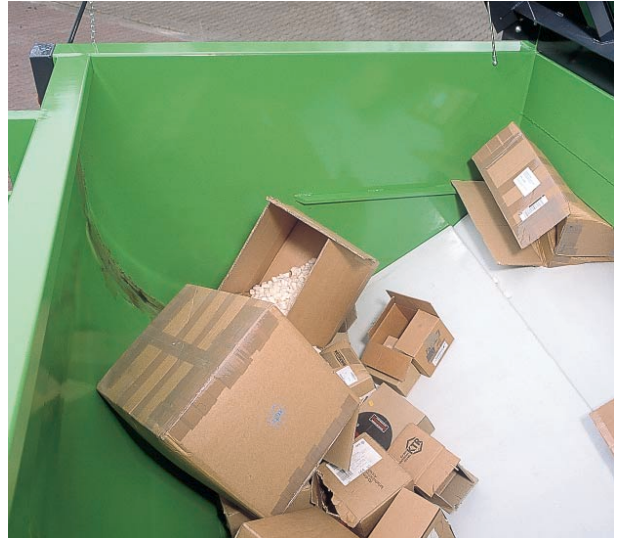
2. During the forward cycle the whole filling area remains available for continuous charging
